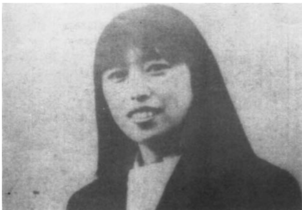
Fig. 1 Light image formation on PAn/TiO 2 film immersed in 0.5 mol dm -3 phosphate buffer (pH 7) containing 20 wt% methanol by projecting the positive image on the PAn/TiO 2 film with illumination by a 500 W xenon lamp for 1 min
